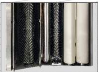
6 Belt cleaning device
